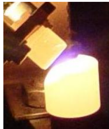
Fig. 2. TVA gun and Be plasma.
